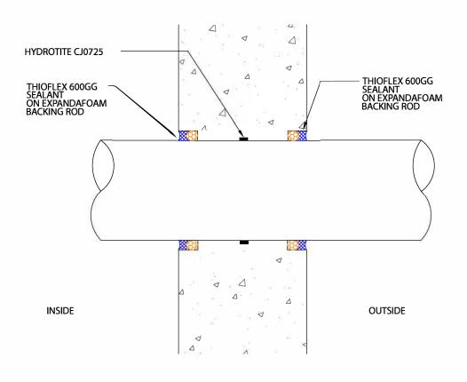
**FUEL PIPE THROUGH WALL DETAIL**
