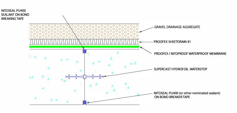
**ROOF CONSTRUCTION JOINT DETAIL**
