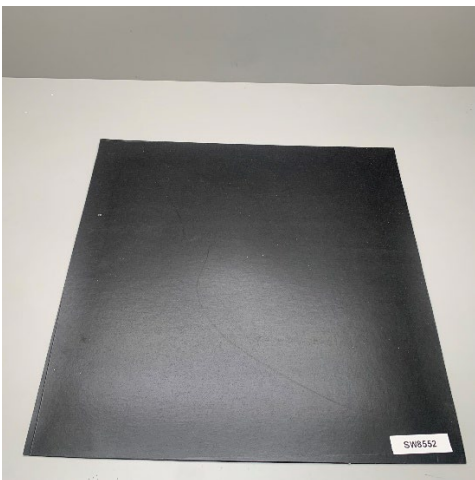
Figure 2 Underside of Nitoproof 610
