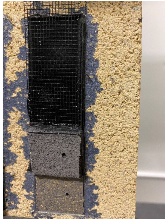
FIGURE 4 IMAGES OF TEST SAMPLE PERFORMING ADHESION-IN-PEEL
