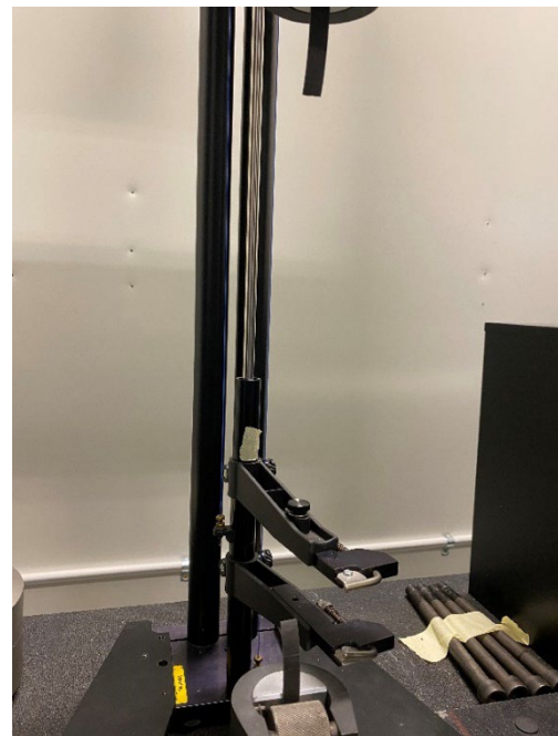
FIGURE 3 IMAGES OF TEST SAMPLE PERFORMING DURABILITY LOAD / ELONGATION TEST
