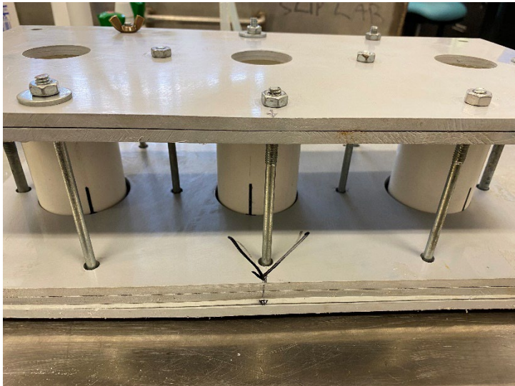
Figure 3 Test apparatus and weighing of Nitoproof 410
