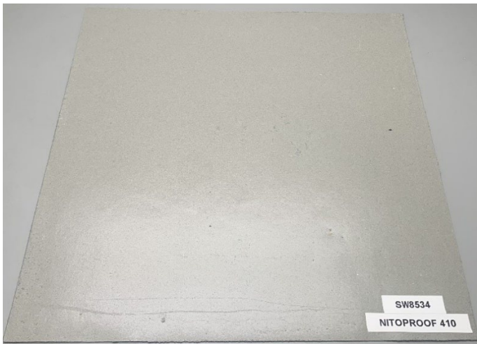
Figure 2 Underside of Nitoproof 410 for SW8534(1st revalidation)
