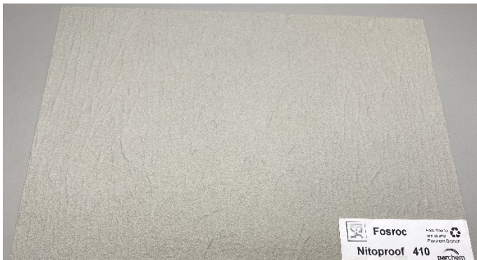
*Top face of Nitoproof 410 for 8363A (the main previous report)
